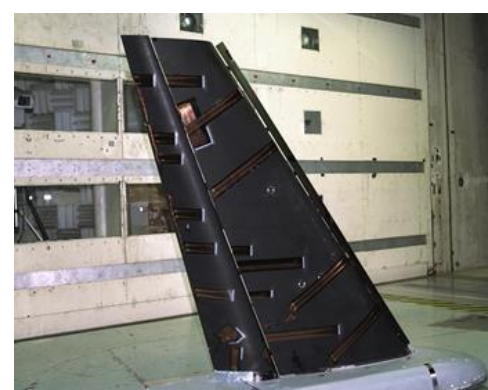
(b) Trap wing in 14-by-22-Ft. tunnel Figure 11-49: The NASA trapezoidal wing.
